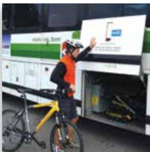
**3** Lift the lever and push the door up, making sure that the door is fully extended. Attach the safety chain by inserting pin in hinge area.
