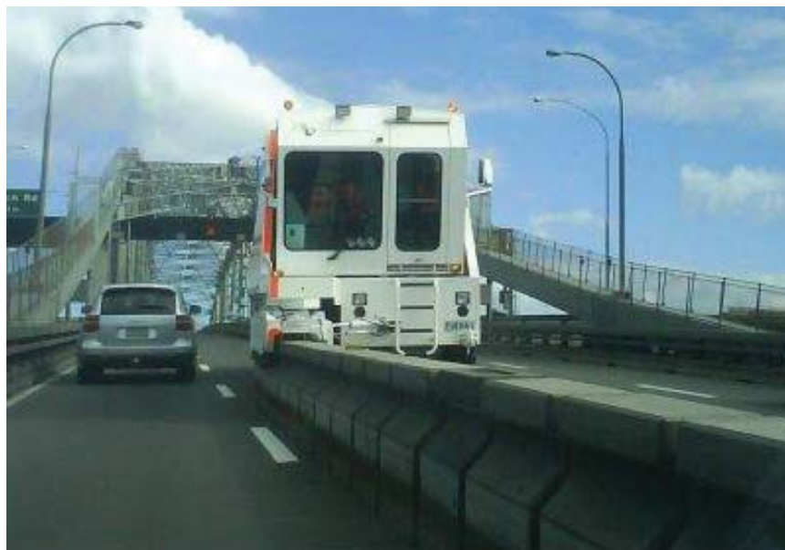
Auckland Harbour Bridge Barrier Transfer Machine
