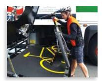
If loading bike onto the upright position (upper skin), be sure to align tires in wheel tray and secure the three straps.
